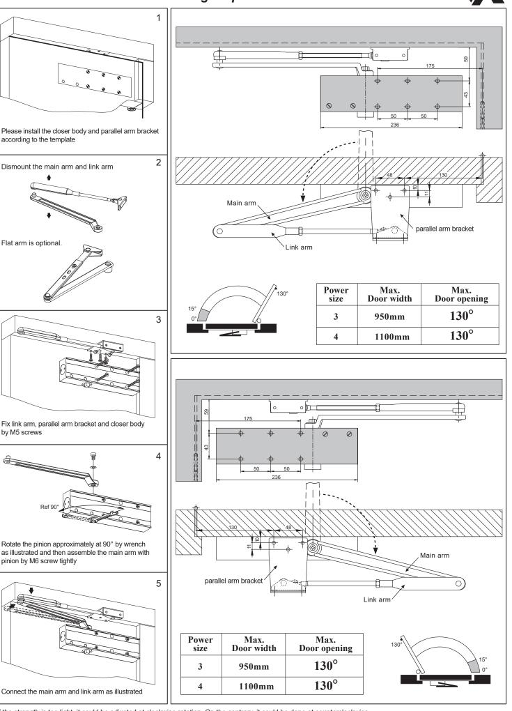
💥 If the strength is too light, it could be adjusted at clockwise rotation. On the contrary, it could be done at counterclockwise.
